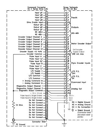
Figure 41: ECI-44 Signal Connections
